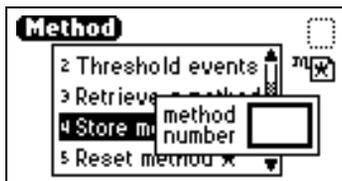
3. Enter a number from 1 to 10 (inclusive), and press Enter. A brief message (“Storing \* as method *n*”) appears. When the display returns to the Method choice list, the method number you selected appears within the method icon. That method remains active until you retrieve another method or reset the detector to default conditions (Method \*).
