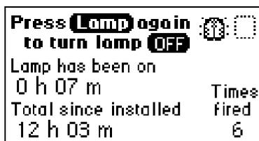
2. Press Lamp (press Shift, 1) again to extinguish the lamp. The Home screen appears with an X through the lamp indicator icon and the words “Lamp off”.
